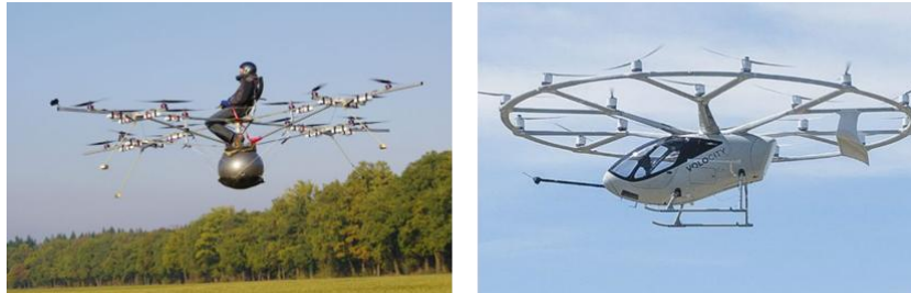
Fig. 5 – Multicopter prototype and current model of Volocopter
