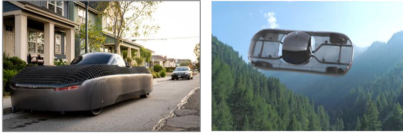
Fig. 15 – Alef ´ s flying car on the road (photo) and in the air (animation)
