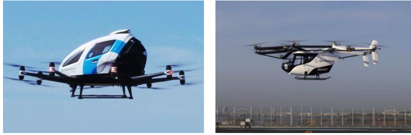
Fig. 6 – Multicopter from Ehang and Skydrive (Source Ehang and Skydrive)
