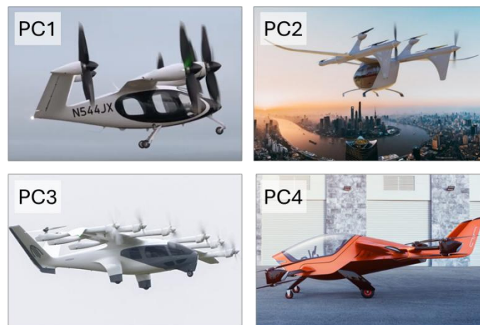
Fig. 9 – Propeller configurations wing-based eVTOL
